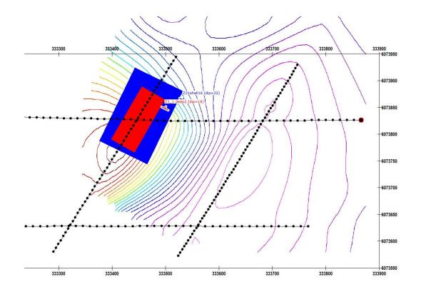
The Z3\_1 anomalies are shown in plan with the gradient removed TMI contoured below. Preliminary inversion of the aeromagnetic data shows the magnetic structure concentrated at the depth of the deep stronger conductor.
