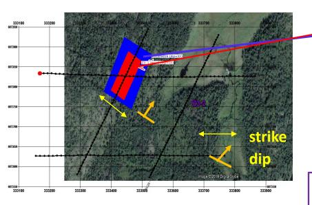
The 2 parts of the model are shown. One shallow, weaker conductor in blue and the deeper, more conducting target in red.
